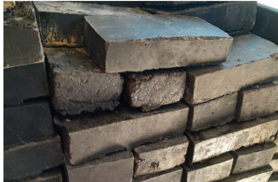
Plastic bricks made from recycled plastic by Moeketsi Motantsi in Lesotho
